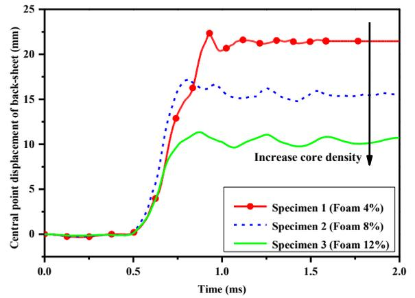
Fig. 4. Time history of backward displacement of structures intended to investigate the effect of the core density
