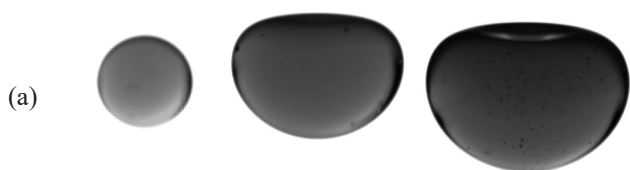
Fig. 3. A comparison between the steady shape of (a) the analytical solution of Taylor and Acrivos [4] (b) the experimental section at k=0.25
