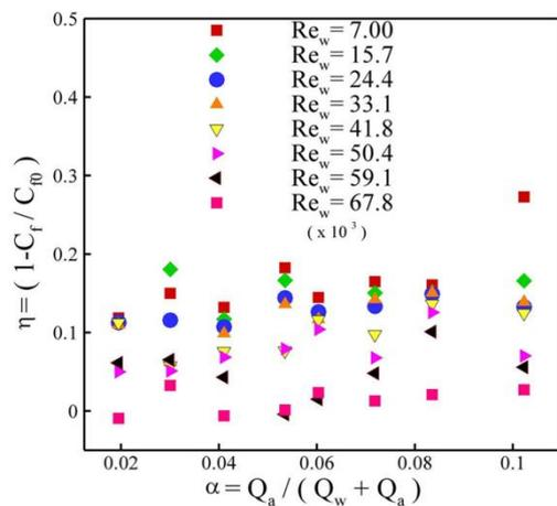
**Fig. 1 Drag reduction ratio changes by increasing void fraction  $\alpha$  in various  $Re_\omega$**
