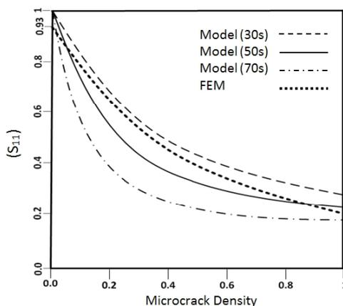
Figure 3. FEM results of three-element model for  $S_{11}$
