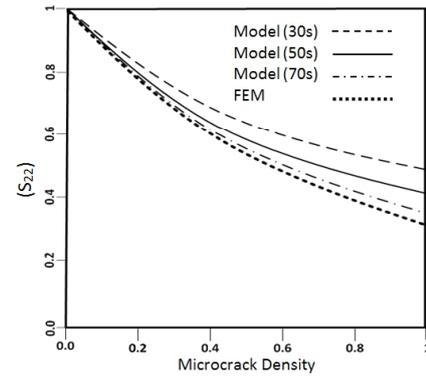
Figure 4. FEM results of three-element model for  $S_{22}$
