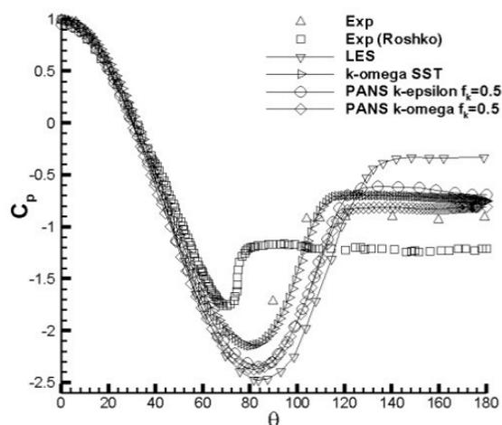
Figure 1. Pressure coefficient curve on the upper half of cylinders
