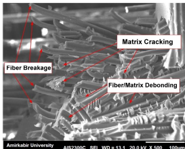
Figure 2. SEM images of damage surfaces of the specimens
