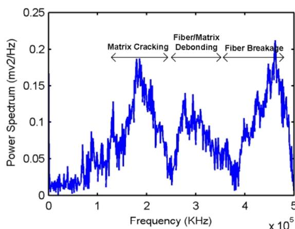
Figure 1. AE frequency spectrum of the specimens
