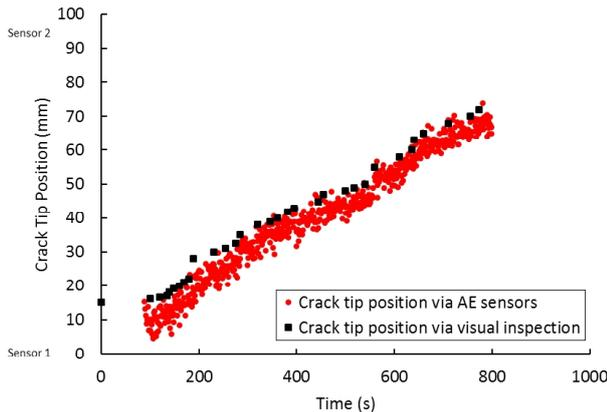
**Figure 3. The predicted crack tip position using AE method versus visual inspection data**
