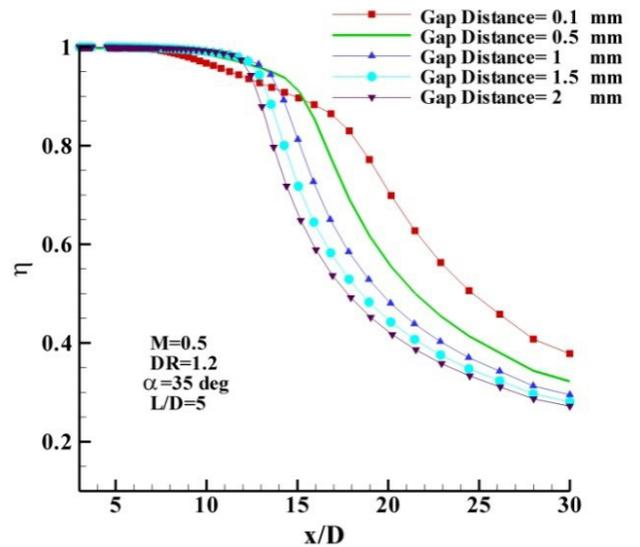
Figure 5. Film cooling effectiveness with different positions of actuator
