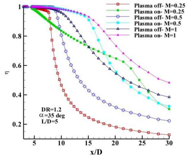
Figure 4. Film cooling effectiveness in different blowing ratios
