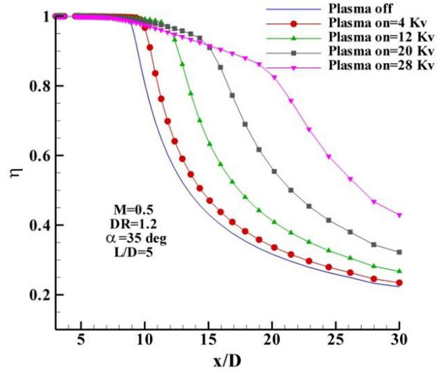
Figure 3. Film cooling effectiveness under different voltages
