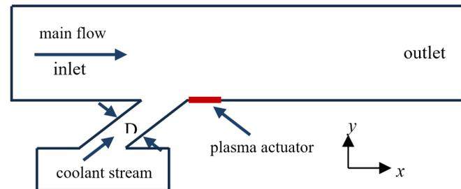
Figure 1. Computational domain geometry
