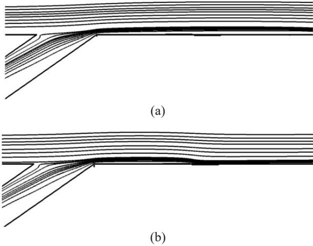
Figure 2. Stream lines from the film hole, (a) without plasma actuator, (b) with plasma actuator
