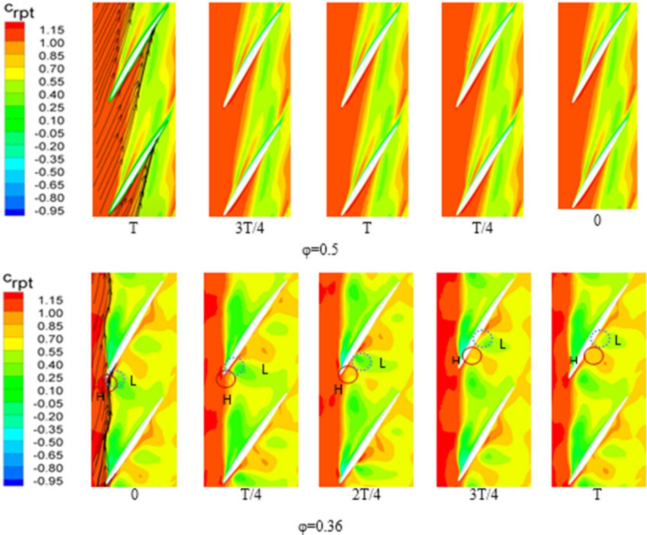
Figure 2. Unsteady fluctuations of static pressures on 97% span stream-surface
