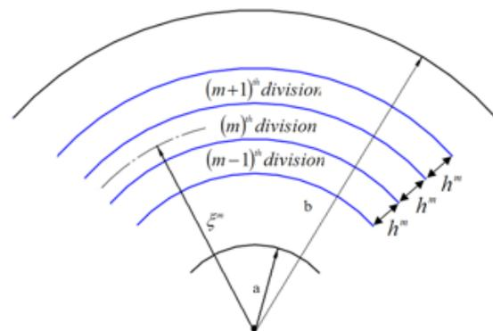
Figure 1. Division of cylinder thickness
