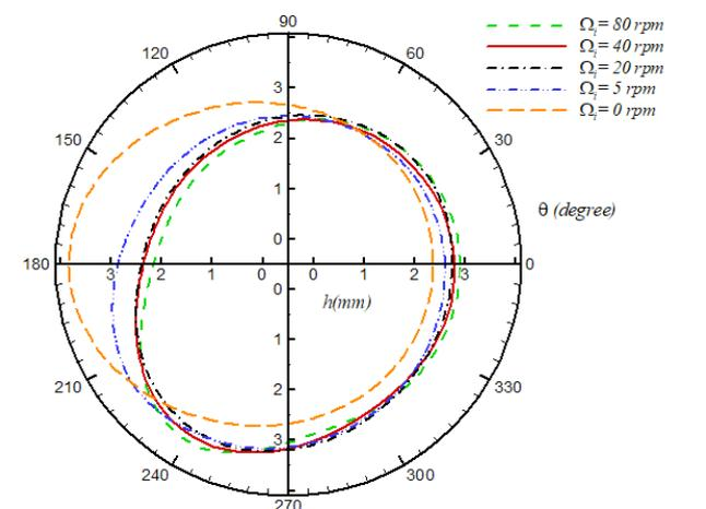
Figure 4. Effect of eccentricity on cake thickness
