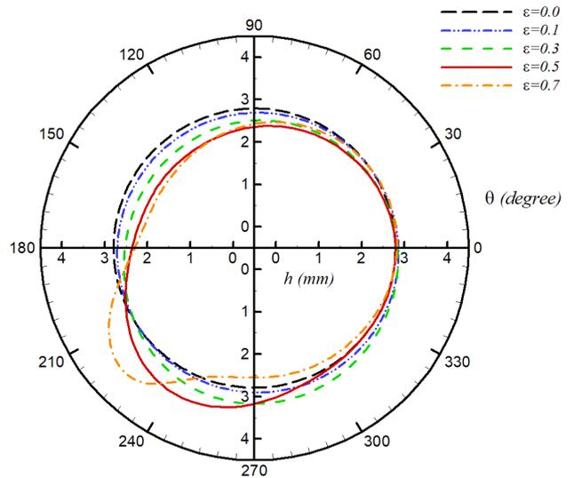
Figure 3. Effect of eccentricity on cake thickness
