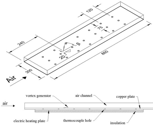
**Figure 1. Schematic sketch of the test section, copper plate, and their dimensions.**
