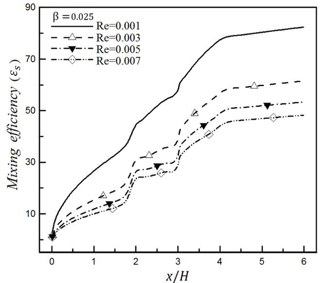
Figure 3. Mixing efficiency changes per specific slip coefficient (0.025) and different Reynolds number for (np-pn) pattern
