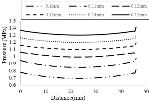
Figure 2. Effect of depth of channel on pressure distribution of GDL
