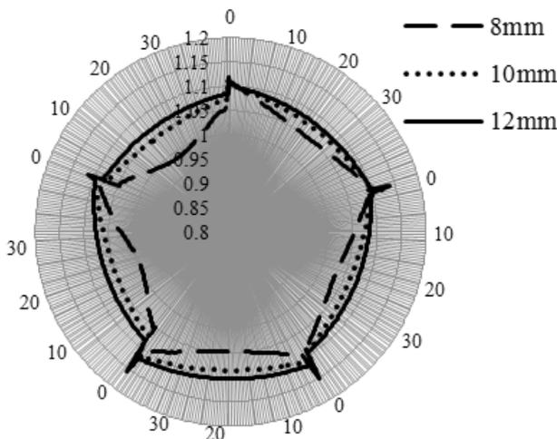
Figure 3. Pressure distribution over GDL for different thicknesses of the end plate.
