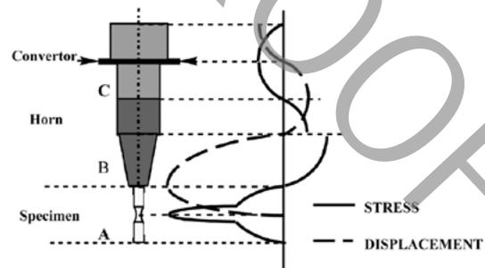
Fig. 1. Displacement and stress distribution [1]
