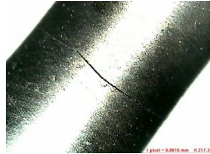
Fig. 4. Cracks grown in a sample that has been photographed with VMM
