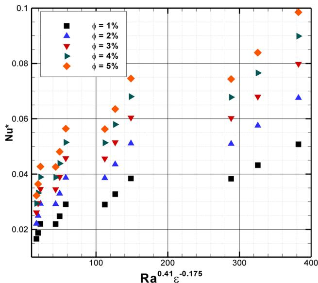
Figure 1. Variation of  $Nu^*$  with nanoparticle size and Rayleigh number for different volume fraction of nanoparticles
