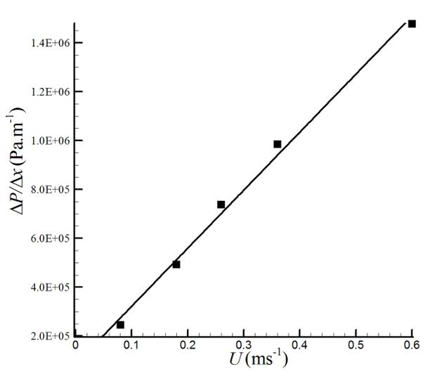
Figure 2. Results of the permeability test
