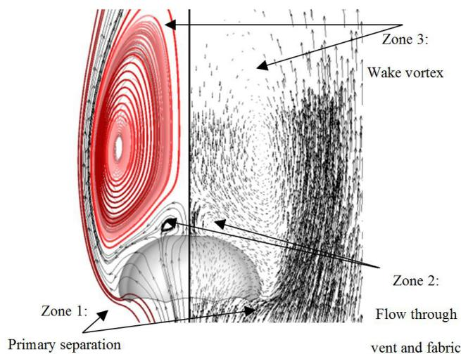
Figure 3. Surface streamlines and vectors around 3D parachute
