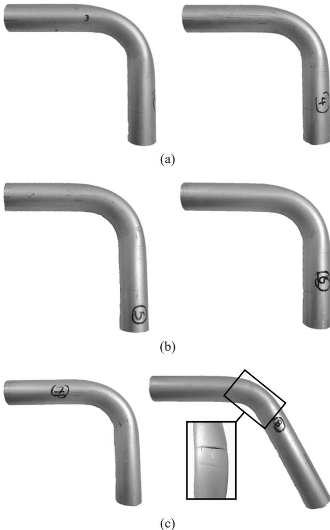
**Fig. 1. Bent tubes at different pressures, (a) 1.5 MPa, (b) 2 MPa, (c) 2.5 MPa, (d) 2.8 MPa, (e) 3.3 MPa, (f) 3.7 MPa**
