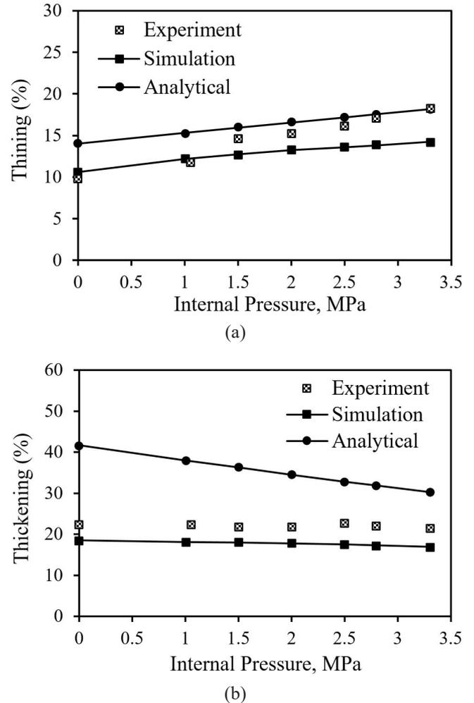
**Fig. 2. The effect of internal pressure on, (a) thinning in extrados, (b) thickening in intrados**
