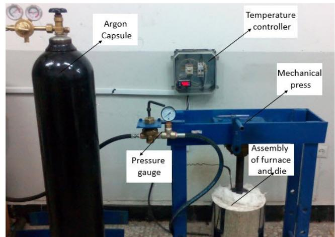
Fig. 1. Overview of experiments setup
