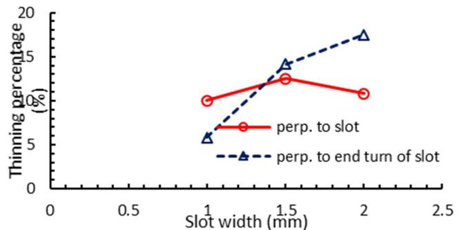
Fig. 7. Comparison of sheet thinning percentage of different widths of the slot in 35 bar, 1000 °C and 10 min
