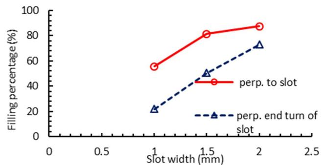
Fig. 6. Filling percentage of different widths of the slot at 1000 °C, 35 bar and 10 min
