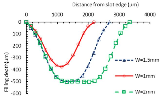
Fig. 5. Comparison of sheet filling profile at 1000 °C, 10 min and 35 bar
