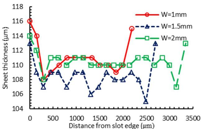
Fig. 4. Comparison of sheet thickness distribution at 1000 °C, 10 min and 35 bar
