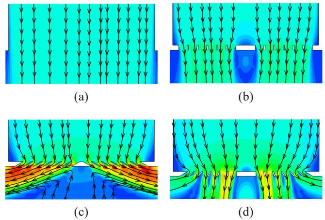
**Fig. 2. Streamline and contour of entering air velocity to the ventilated room of a) W/O diffuser, b) 90°, c) 30° and d) 30-90 degree diffuser angle**
