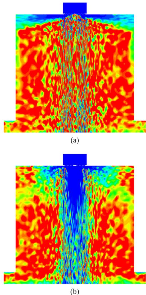
**Fig. 3. Contaminant concentration contour at time 10s in the configuration of a) 30° and b) 30-90 degree diffuser angle.**
