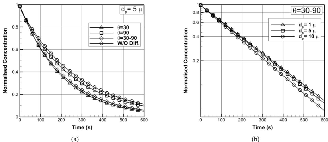
Fig. 4. Normalized concentration versus time of (a) different configurations; (b) different particle diameters
