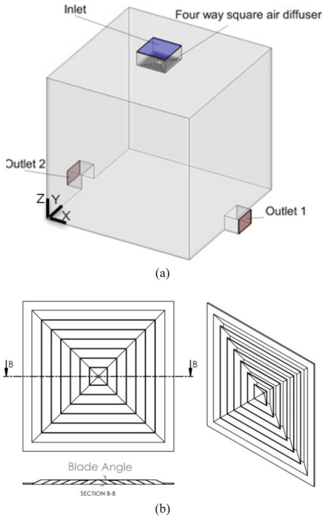
**Fig. 1. Geometry of (a) ventilated room (b) Four way ceiling diffuser**
