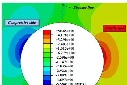
Fig. 2. Circumferential stress contours around the notch border (0.3-2-50)
