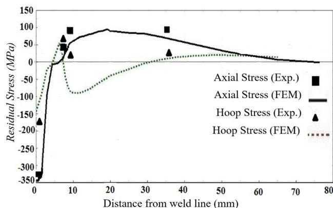
Fig. 4. Hoop residual stress distribution on the inner surface of the pipe for three different filler with 1500 J heat input
