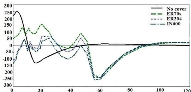
Fig. 6. Hoop residual stress distribution on the inner surface of the pipe for three different fillers with 3000 J heat input
