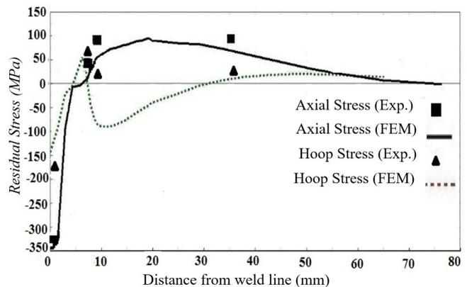
Fig. 2. Comparison of axial and hoop residual stress distribution in the finite element model and experimental sample on Outer Surface
