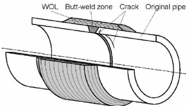
Fig. 1. Overlay welding [1]
