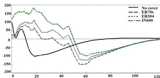
Fig. 5. Axial residual stress distribution on the inner surface of the pipe for three different fillers with 3000 J heat input
