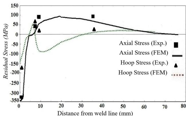
Fig. 3. Axial residual stress distribution on the inner surface of the pipe for three different filler with 1500 J heat input
