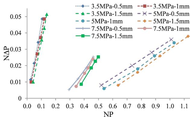
**Fig. 8. The differential pressure versus pressure drop rate for different initial pressures and orifice diameters (non-dimensional)**
