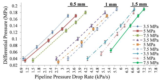
Fig. 7. The differential pressure versus pressure drop rate for different initial pressures and orifice diameters
