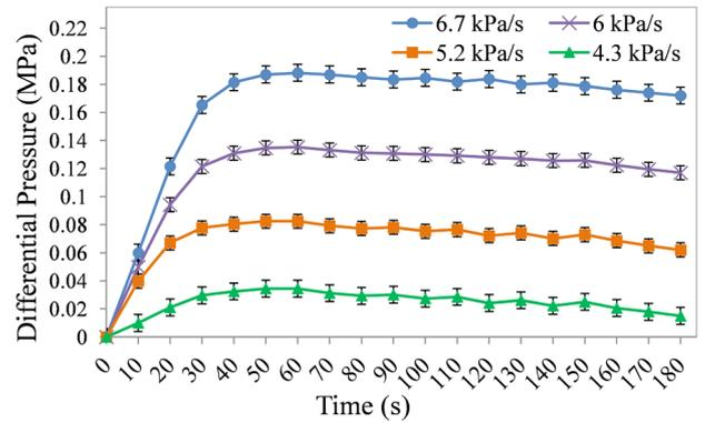
Fig. 6. The differential pressure versus time for  $P_i=3.5$  MPa and orifice diameter of 1.5 mm
