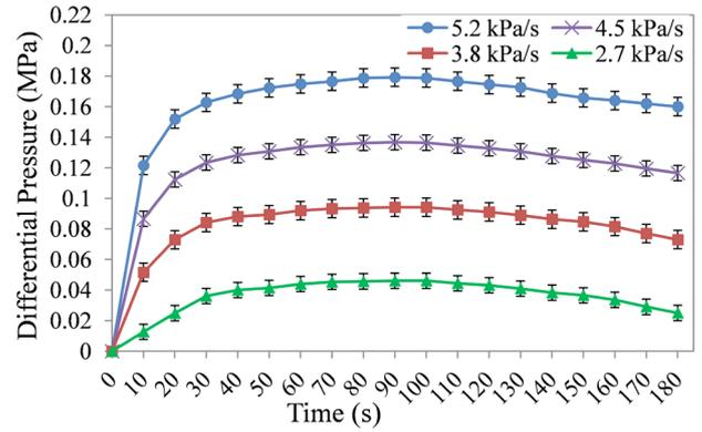
Fig. 5. The differential pressure versus time for  $P_i=3.5$  MPa and orifice diameter of 1 mm
