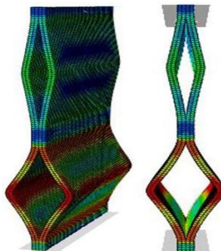
Fig. 21. Schematic diagram of double cells absorber collapse in both front and isometric views at the end of time intervals
