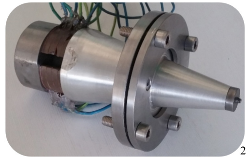
Fig. 6. 1- Detached parts of ultrasonic transducer and tool set, (1. FSW tool insert, 2. Concentrator, 3. Backing, 4. Copper electrodes, 6. Stud bolt)
