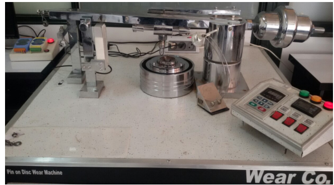
Fig. 4. wear device of pin on disc
