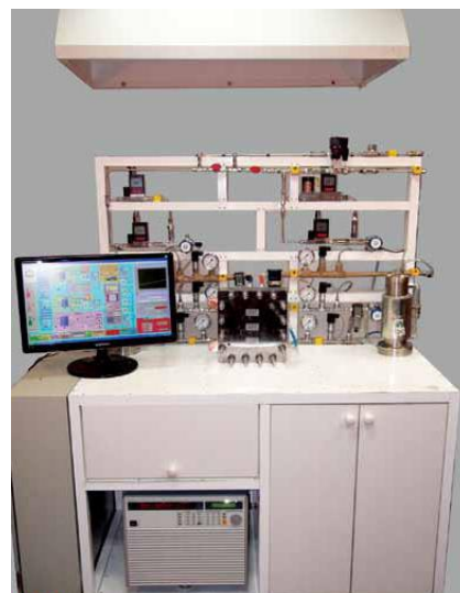
Fig. 9. A view of the stack and single-cell test system for polymer electrolyte membrane fuel cell
