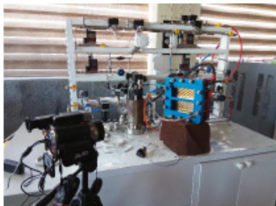
Fig. 3. Fuel cell testing system along with the thermal camera
