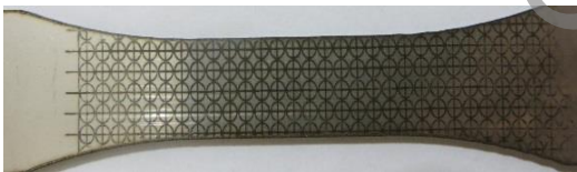
Fig. 5. Final specimen graphed with electrodes
