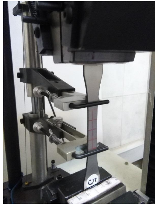
Fig. 12. Specimen under stretch test in Santam STM-20 machine
