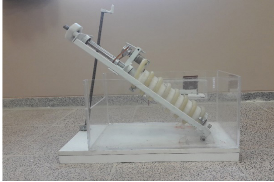
Fig. 1. Rotating helical pump
