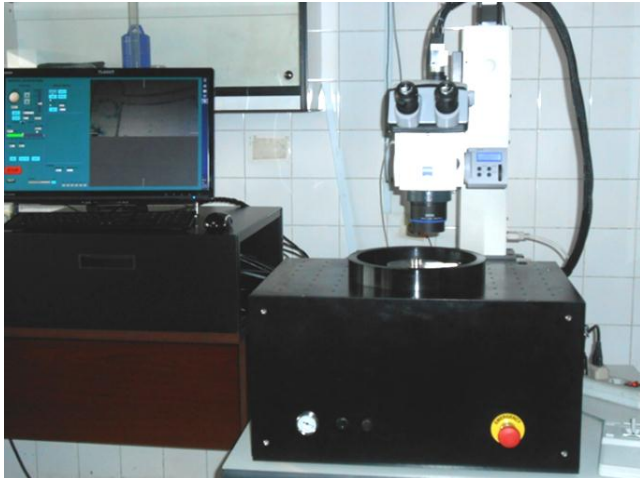
Fig. 5. Testing machine for microfluidic discs
