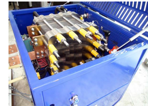
Fig. 5. Integrated power system for dead-end tests
