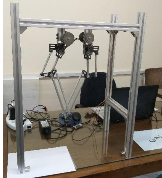
Fig. 2. The 2-DOF parallel robot with two adjustable counterweights
