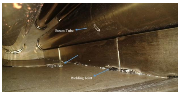
Fig. 1. The location of welding joints on the flight bars
