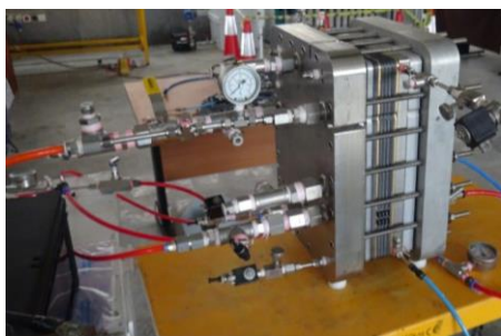
Fig. 1. The PEM fuel cell with integrated humidifier
