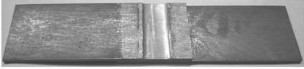
Fig. 1. The resulting welded specimen
