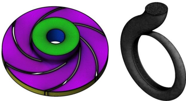
Fig. 2. The grid generated for the impeller and volute
