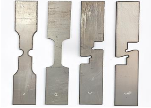
Fig. 1. Two sheared samples, Dog-bone and grooved specimen.
