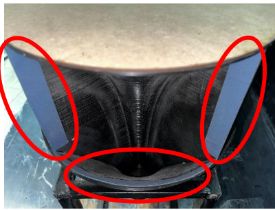
Fig. 2. Place of surface roughness at the inlet
