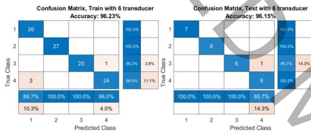
Figure 2: Confusion matrix of the proposed ensemble model for the train data (left) and the test data (right)
