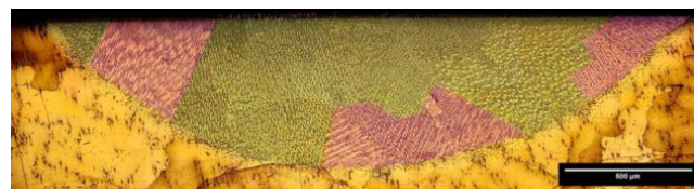
Fig. 2. The formation of equiaxed dendrites in the upper regions of the pool, shown in green, and the growth of columnar dendrites in regions close to the fusion line, shown in pink.
