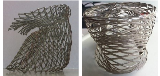
Fig. 2. Collapse of tubes with cell angle \alpha=0 and \alpha=90
