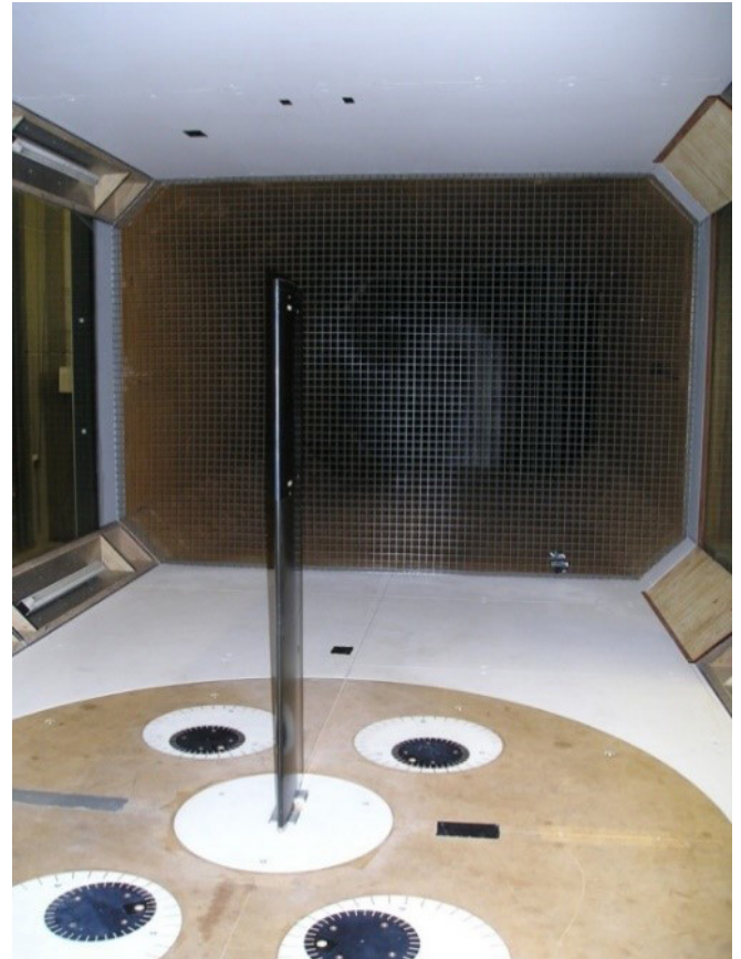
Fig. 1. Installed model in the wind tunnel test section
