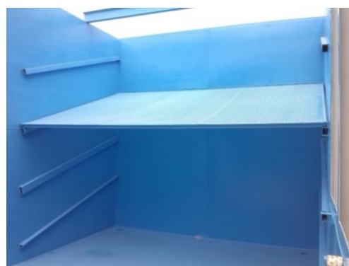
Fig. 5. The damper system of wave tank
