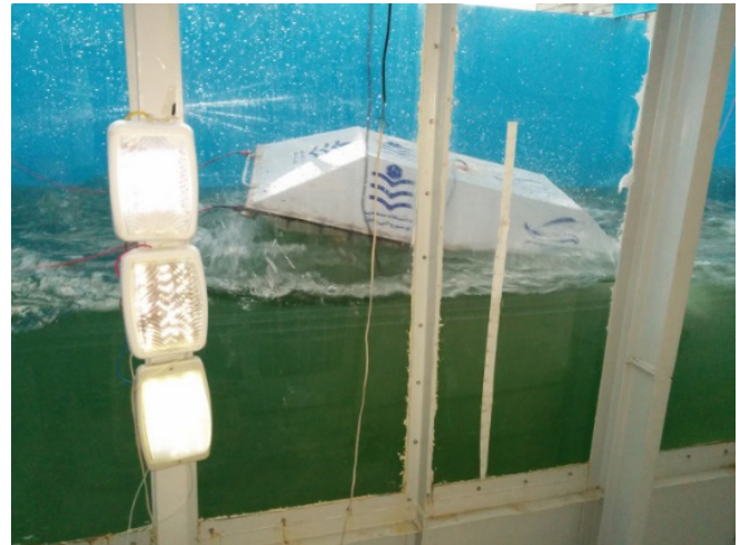
Fig. 11. The WEC with lamps in the test system
