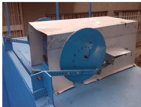
Fig. 4. Motor and moving mechanism of the paddle
