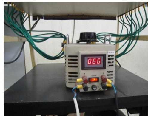
Fig. 4. Source of low voltage generator
