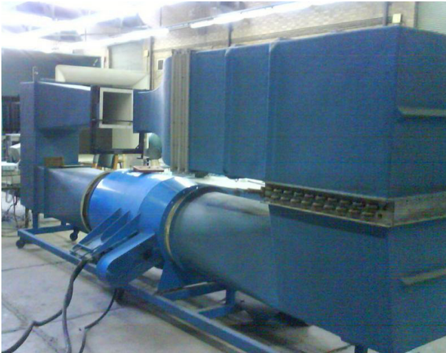
Fig. 4. The wind tunnel used for calibration
