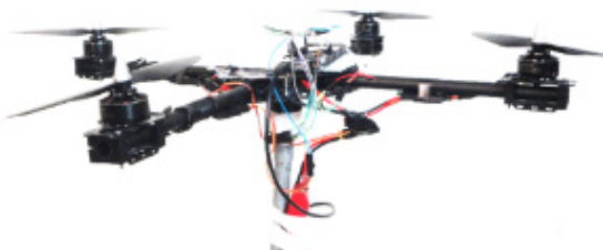
Fig. 3. Quadrotor on the base with three degrees of freedom
