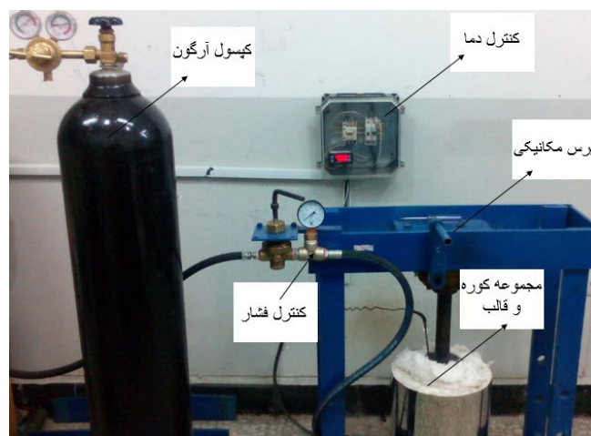
Fig. 1. The photograph of the die set
