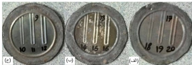
Fig. 6. The formed sheets at pressure a) 15, b) 25 and c) 35 bar
