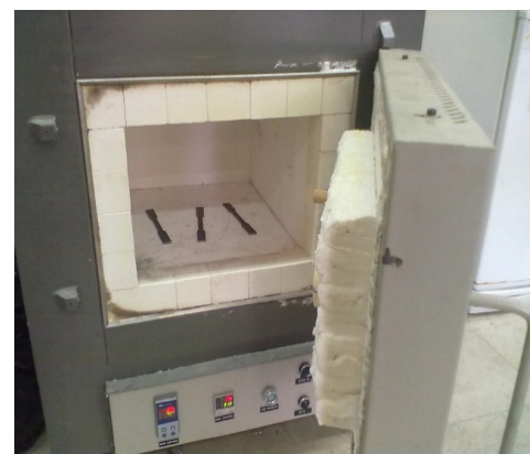
Fig. 6. Stresses relieving of the test samples by heat treatment.
