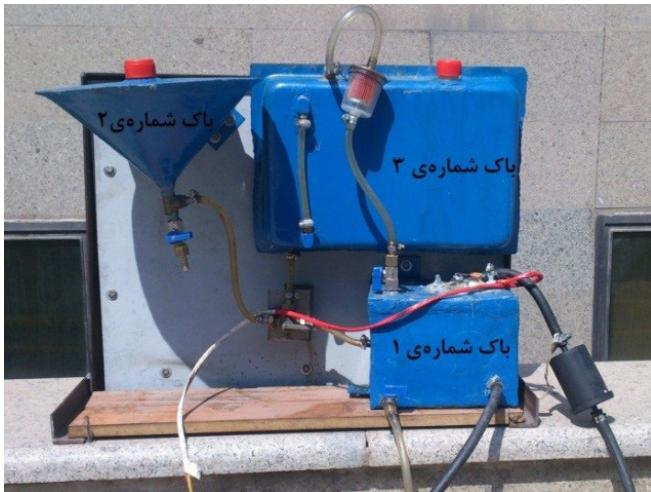
Fig. 6. The fuel consumption measuring device
