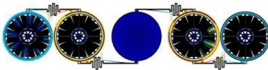
Fig. 4. Demonstration of in-plane vibration of the sensor at f = 16.5 kHz
