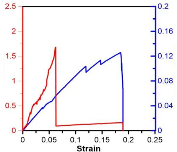
Fig. 2. Electromechanical performance (stress-strain diagram and GF characteristics) of an auxetic sensor
