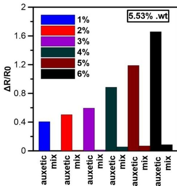
Fig. 1. Comparison of performance of conventional and auxetic sensors made with a mixture of silicone rubber and chopped carbon fibers.
